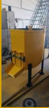
Tower Crane Concrete Bucket
