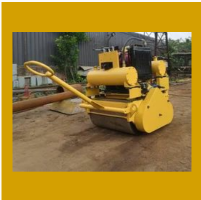
Vibratory Soil Compactor
