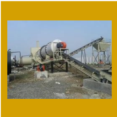
Asphalt Hot Mix Plant
