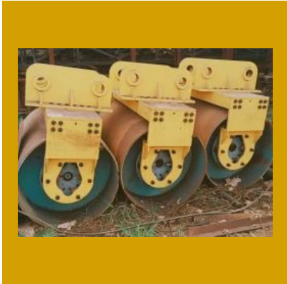
Railway track extension compactor
