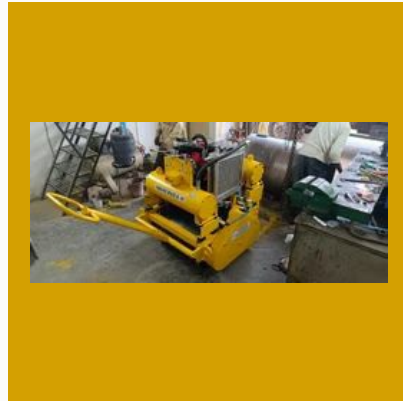
Vibratory Soil Compactor
