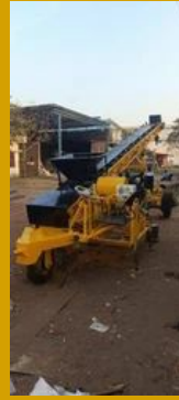
Mobile Conveyor concrete
