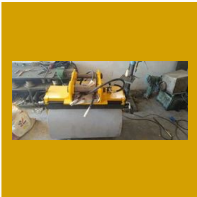
Slope Compactor Rollers
